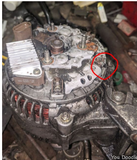
The lug pictured is the W+ terminal
